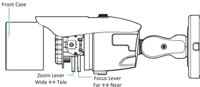
❗ **NOTE** : If the front cover is cross threaded or not correctly tightened the camera housing will not be weatherproof.
