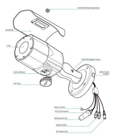
Before installing your camera, you have to read the following cautions. 1. You have to check whether the location can bear five times of the weight of your camera. 2. Don't let the cable to be caught in improper place or the electric line cover to be damaged.
